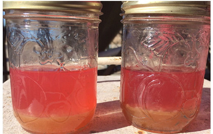
Contaminated Diesel Fuel
